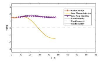
Fig. 5. Two hypothesis trajectories: lane keep and lane change for a vehicle traveling on a two lanes road.
