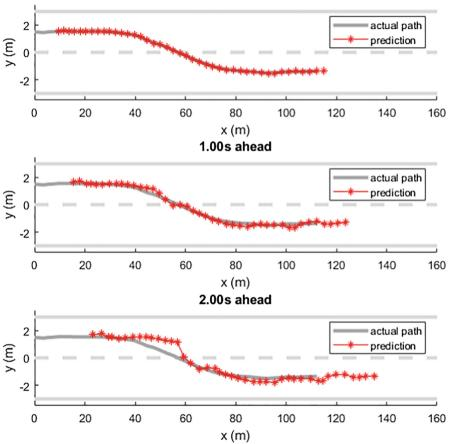
Fig. 6. Predicted trajectory for different look ahead times: 0.25 s, 1 s and 2 s. The thick grey line shows the actual path.
